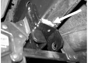
**STEP 1B:** With a cleaning solvent, clean the area where the END LINK BRACKET will be located.
