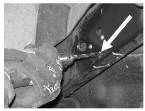
**STEP 1F:** With the END LINK BRACKET off the chassis tube frame and the three holes drilled out to 3/8", insert the nut-serts supplied with the kit (there should be a total of 10 in the kit) (See Parts List). With the nut-sert, nut sleeve and bolt assembled, push the nut-sert into the holes, making sure they are flush to the chassis tube frame.
