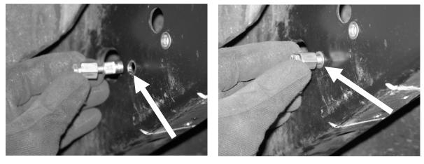
**STEP 1G:** To lock the nut-sert in place in the chassis tube frame, using a 7/16" wrench or a ratchet with a 7/16 socket head (bolt) and a 1/2 wrench (nut sleeve), begin tightening the bolt. The knurl end of the nut-sert locks into the thickness of the chassis tube frame, while the end expands on the inside. Tighten until you are not able to turn it anymore, just stopping short of not being able to turning it. Do this for all three holes that have been just drilled.
