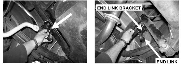
**STEP 3B:** The simplest way to install the new Anti-Sway Bar is by mounting the ends of the Sway Bar to the ends of the end links. Begin by attaching one end at a time. Using an adjustable jack stand to help in supporting the Anti-Sway Bar, hold one end up to the end link and insert the mounting hardware. Do this to both ends.
