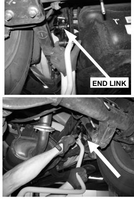
**STEP 3C:** Tighten both hardware to torque specs.
