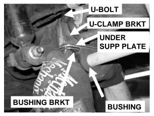
**STEP 3G:** Using a 9/16 wrench or a ratchet with a 9/16 socket head, tighten and lock down the mounting hardware.
