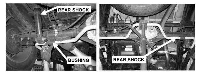
**STEP 3F:** Slide the U-shape mount screw over the top of the rear axle, with the legs pointing downward. The U-CLAMP bracket will face up with the legs facing upwards. The UNDER SUPPORT PLATE will locate between the UNDER SUPPORT PLATE and the back of the BUSHING. The BUSHING BRACKET will slide over the BUSHING mating up with the U-CLAMP.
