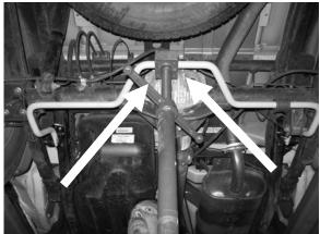
**STEP 3E:** Locate the drivers side bushing near the inside of the rear shock. The passengers bushing near the inside of the rear shock.
