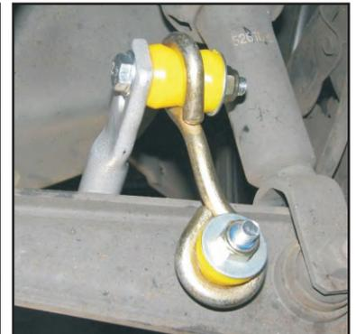
Photo 3. Link assembly - front view.
